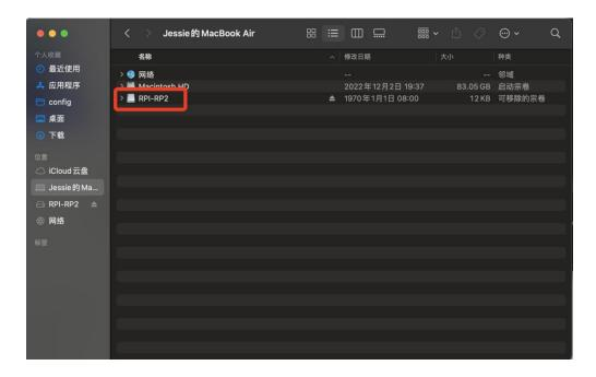
Download <u>rp2040 uf2</u>, copy the .uf2 file in the firmware package to the disk, then the disk will log out.
