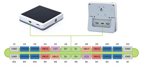
Note: A2, A3, A10, A11, B2, B3, B10, B11 connect to RP2040 GPIO8, GPIO9, GPIO0, GPIO1, GPIO2, GPIO3, GPIO15, GPIO14
